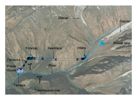
Figure 3: Schematic diagram of a run-of-the-river hydroelectric project.
