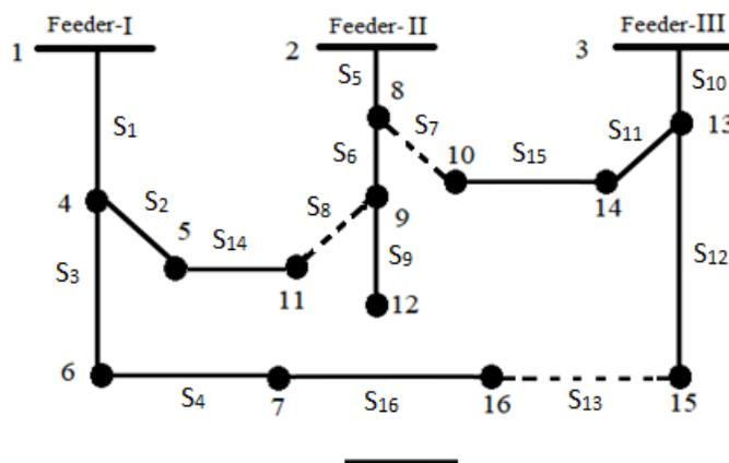
Figure 2: IEEE 3-feeder system after reconfiguration
