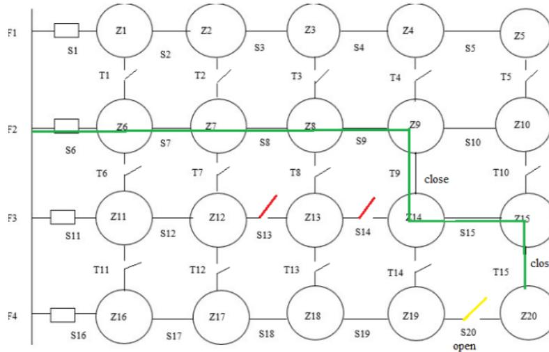
**Figure 5:** IEEE 4-feeder system after reconfiguration
